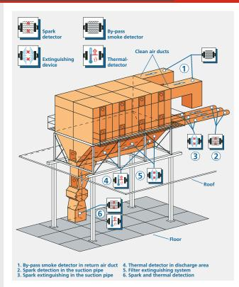
Protection of a Hose filter systems: All suction pipes leading to the filter system are monitored by spark detectors (2) and protected by spark extinguishers (3). If a filter pipe starts smouldering, the alarm is actuated immediately by by-pass smoke detectors (1) in the clean air ducts. Fires due to self-ignition in the filter system are detected by thermal detectors (4) an the alarm given immediately, so that the filter extinguishing system (5) is also activated.
